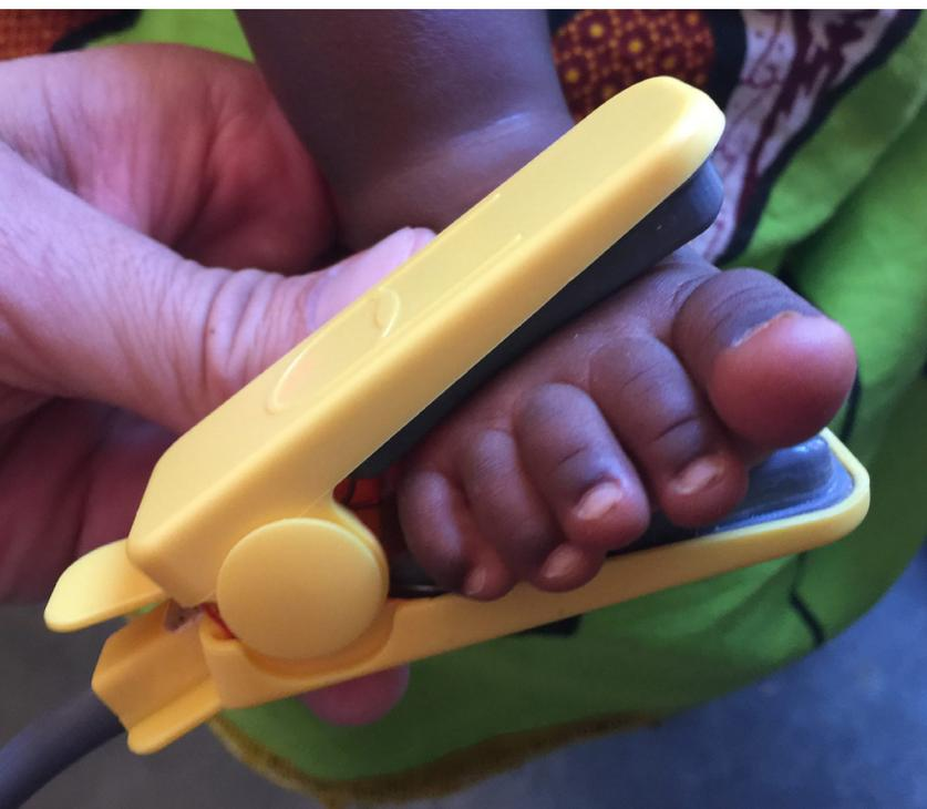
Lifebox, with support from the Bill & Melinda Gates Foundation, has developed a pediatric probe, and made the design available open access, to improve use of pulse oximeters in children.<sup>(25)</sup> Lifebox and Smile Train will, together, continuously seek ways to develop and improve our pulse oximeter technology to meet the needs of all patients.
